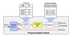
Figure 4: The layout of NetGVT switch data plane.
